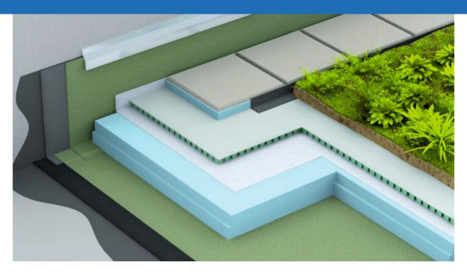
**TIKIDAN GREEN ROOF SYSTEMS** are complete waterproofing and insulation solutions topped with a natural planted surface. This garden surface minimises absorption of the thermal enclosure, thus helping buildings achieve both an energy savings and respect for our environment.
