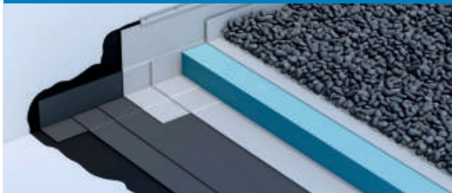
NON-WALKING INVERTED ROOF
