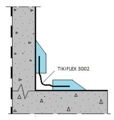
Sealing of a 90° Construction Joints
